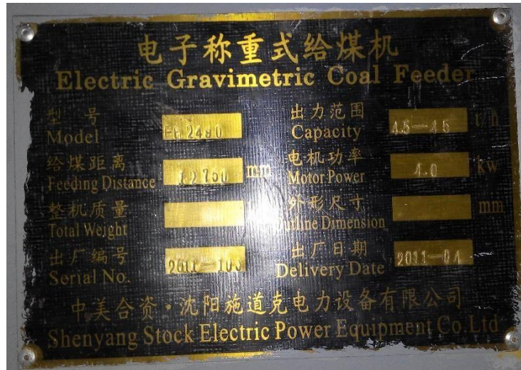
Figure 3.4 Specifications for Coal feeder PLTU Teluk Sirih
